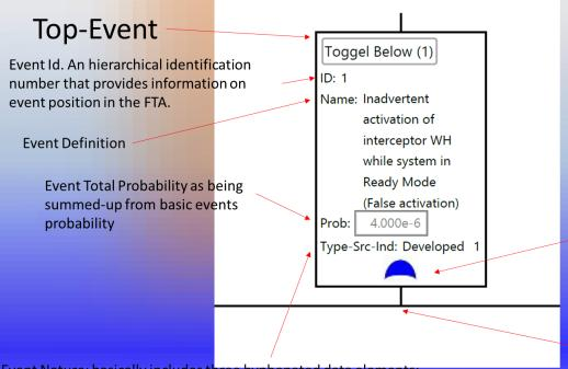
A symbol of the gate through which this event can be generated. This gate may encapsulated OR gate or AND gate where OR gate denotes that at least one of the consequents of events below is required to generate the subsequent events.
